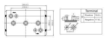
Note: Terminal Torque Values in-lb(Nm):176-203(20-23)
